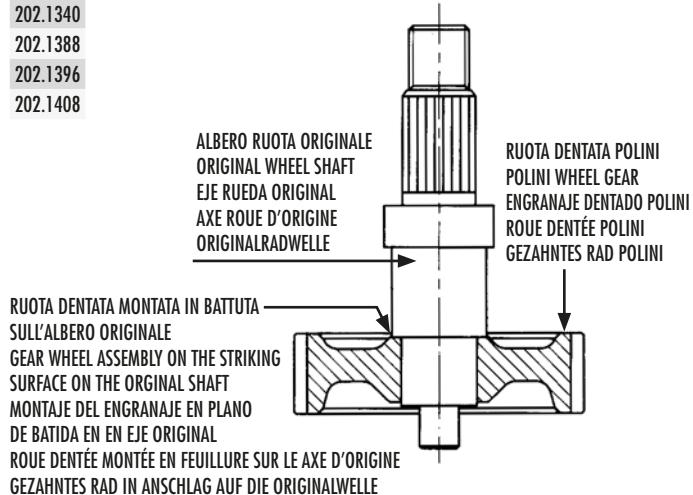
202.1389 ESEMPIO MONTAGGIO DI ALBERO CON BATTUTA - EXAMPLE: ASSEMBLY OF THE GEAR ON THE STRIKING SURFACE - EJEMPLO DE MONTAJE DEL ENGRANAJE EN PLANO DE BATIDA
